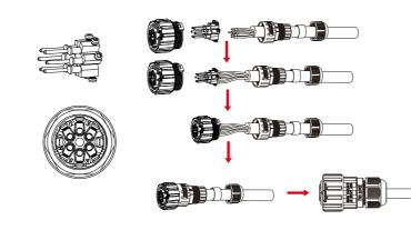
2. Install the waterproof component and screw on the waterproof sheath nut 3. Open the external CT wiring port, the arrow points to the direction of the power grid, put the wire into the external CT card slot, and buckle the buckle.
