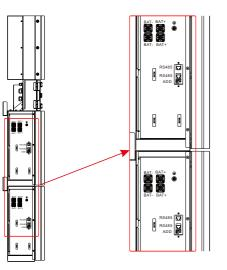
Step 9 Connect the power cables of the bottom battery from Step 4 to the side terminals of the top battery. Make sure that red connects to red and black connects to black.
