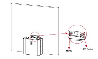
Step 5 To assemble the second (and all other) battery, repeat steps 6 and 7, respectively.
