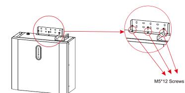
Step 3 Position the battery parallel to the wall and use a \$\Phi 8mm drill to drill holes at a depth of about 70mm in the wall for subsequent fixation of the mounting plates.
