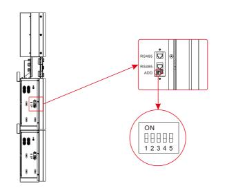
Step10 Open the front cover of the last battery and remove the DIP cover. Now set the DIP switch 2 to "on" mode and close the cover again.
