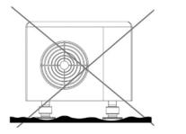
When the weight distribution of the installation is evenly distributed, it is enough to divide the gross total weight by the number of dampers to determine the correct type.
