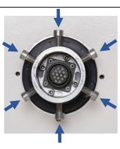
4. Connect the power and data cable from the power box to the camera.
