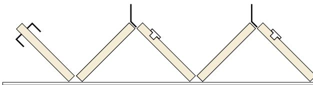
Use one exterior handle on each pair of doors (inswing system) to pull open and close doors.
