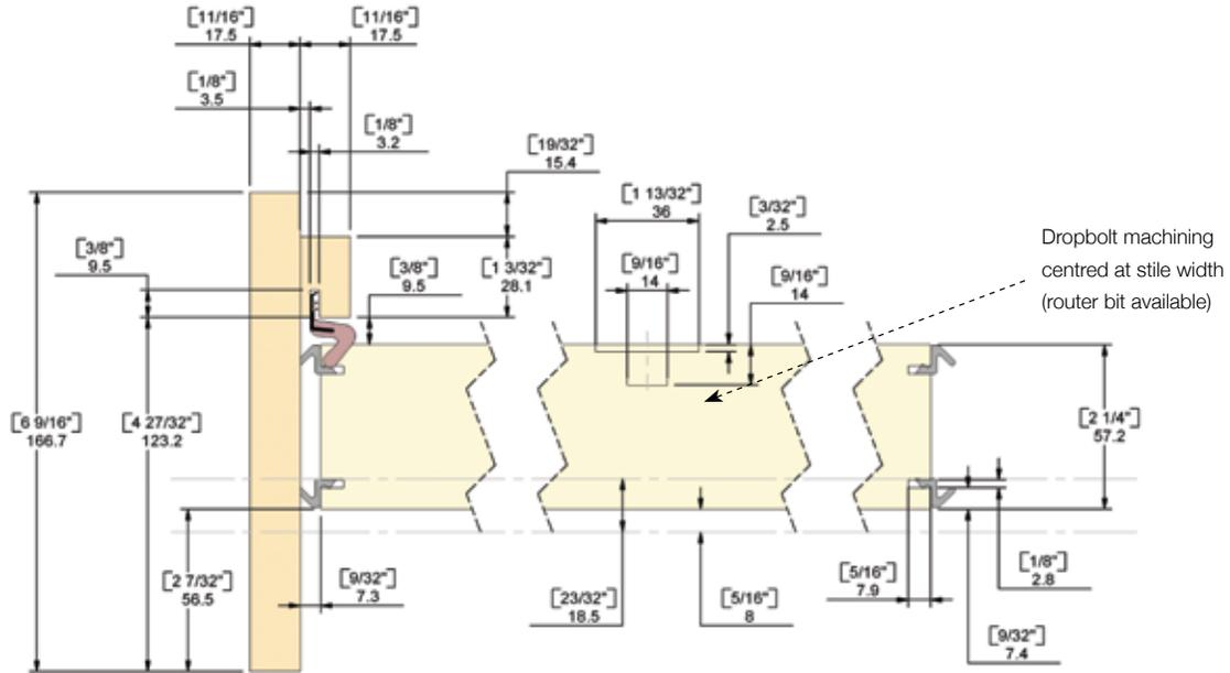
E3 Jamb for 1-3/4" (44.5mm) door thickness
