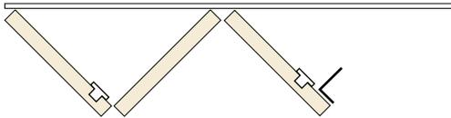
Use one exterior handle on exit door (outswing system) where passage set / lock not required. Use dropbolts top and bottom to lock door from the inside only.
