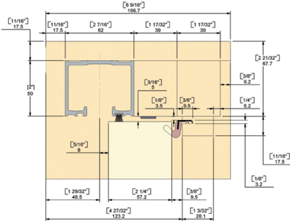
E3 Header for 1-3/4" (44.5mm) door thickness
