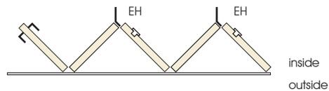
Use one exterior handle on each pair of doors (inward system) to pull open and close doors
