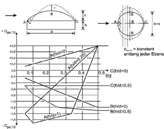
The following coefficients were determined on the basis of these drawings, taken from the standards. They were then applied to the shape in a reasonable way.
