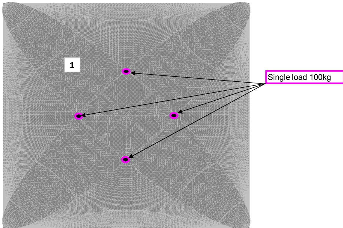
The loading is spread equally on all 4 points. Unequal induction of the loading is impossible.
